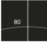
The white number shown half-way between the plane's position and the top of the compass is the range and it represents the distance from the center of the circle to its crossing line.
