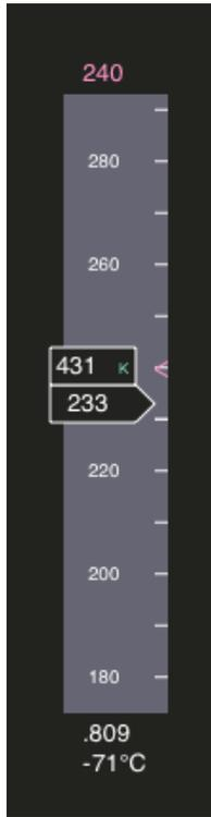
Just to the left of the Attitude Indicator is the Speed Tape and as the name suggests, this section represents speed.
