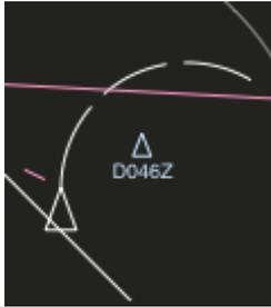
The snake is the arc shown on top of the plane symbol and represents rate of turn.
