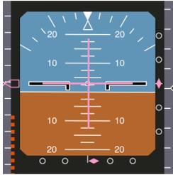
With flight simulator sources two flight-director magenta lines (one vertical and one horizontal) represent the desired flight path.
