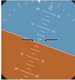
The attitude indicator is in the centre of the PFD, showing the instant roll and pitch angles. The line between brown and blue is the horizon.
