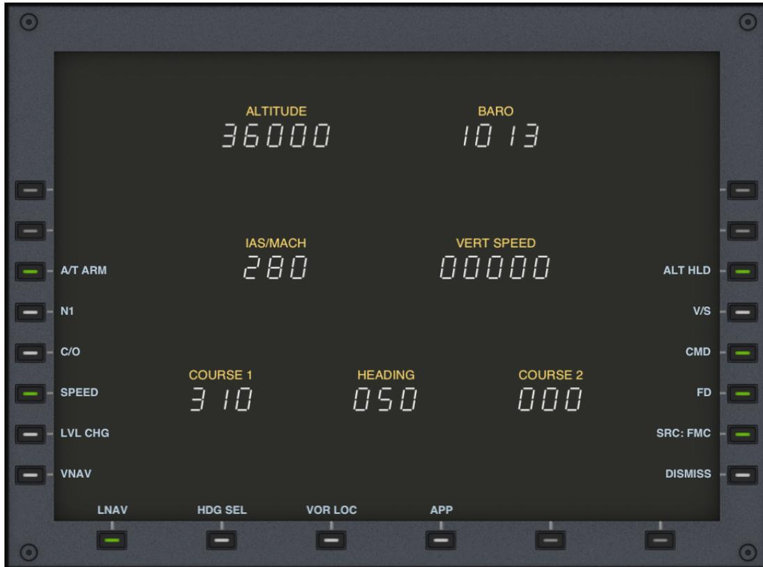
The MCP interacts with the auto-pilot of a flight simulator; it has no purpose when used with Device Location Services other than changing the position of the magenta needles and indicators on the PFD and MFD.
