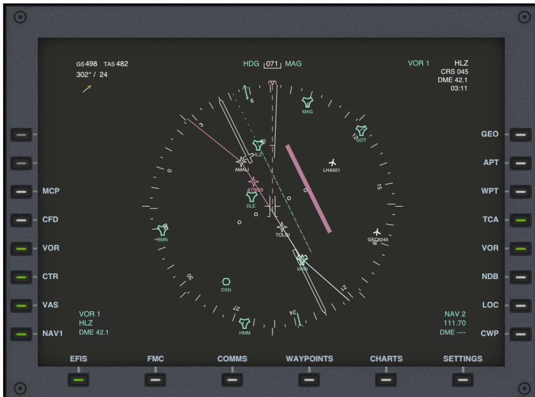
Its frequency, 117.30 Mhz, has been tuned in NAV1 and we are in range, so the radial out of HEC is drawn in green. Because OBS1 was set to 045 degrees, the direction of the radial is 045.
