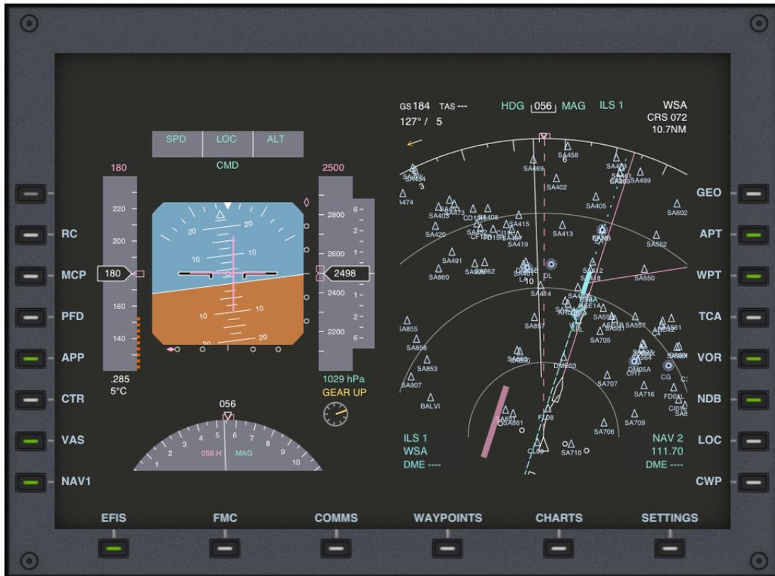
Again the magenta needle moves towards the centre as we capture the ILS direction which is given by the green line. The extend of the green line determines the localizer range, typically 18nm.
