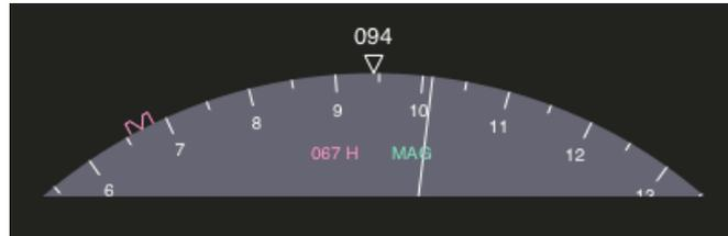
The number on top is the current heading in degrees. The white triangle bug is always on the top just below it.
