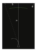
When climbing or descending, the green arc shown represents the point at which the MCP altitude will be reached based on the current vertical and ground speeds.
