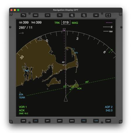
The radial to the VOR is identified as 244; rotate COURSE 1 to 244 so it becomes in line with the radial and switch to APP mode.
