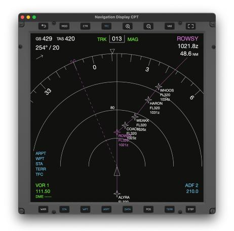
The control buttons on the top and bottom rows act on the respective EFIS panel. In the centre screen there is a navigation map or HSI.
