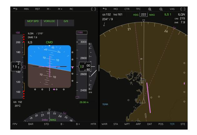
When fully aligned the following screen illustrates the position of the needles. And that's it, touch down soon.
