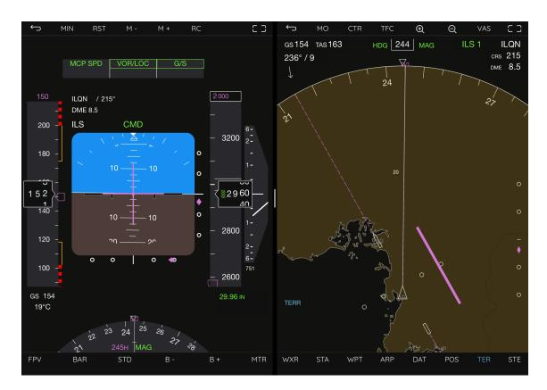
Notice also the position the side magenta diamond which keeps in the middle meaning it is in line with the glideslope.
